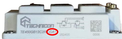
Fig. 2. IGBT C2 case with BIN A1 group marking
